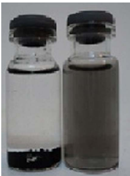
Figure 1. Acetic acid-added aqueous solutions of the CH-wrapped CNTs (right) and the pure CNTs (left). [Color figure can be viewed in the online issue, which is available at wileyonlinelibrary.com .]
